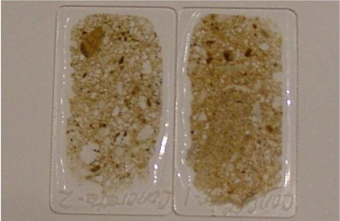
Plate 3 Prepared slides of concrete sample showing heterogeneous distribution of aggregate.
