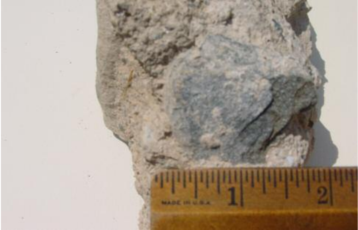
Plate 5 Mica schist aggregate visible in concrete sample from the St Francis Dam.
