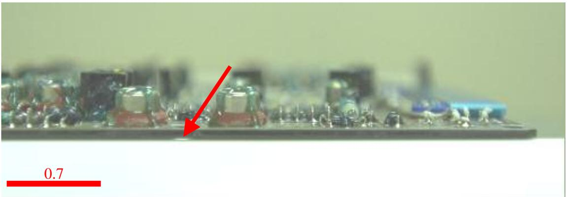
**Figure 3-5:** This photo shows the area where the measurement was taken for the board flatness assessment.
