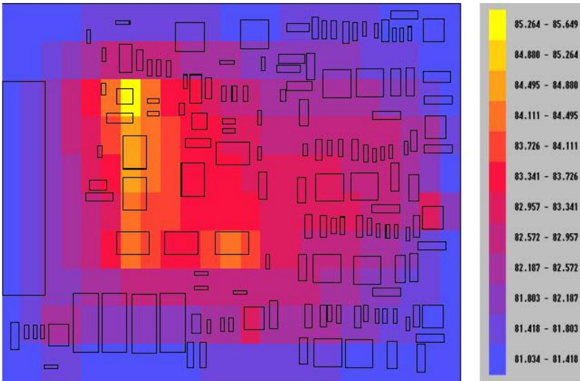
**Figure 6-5: Temperature distribution across Electronics Interface (SPA) at  $81^{\circ}\text{C}$ .**
