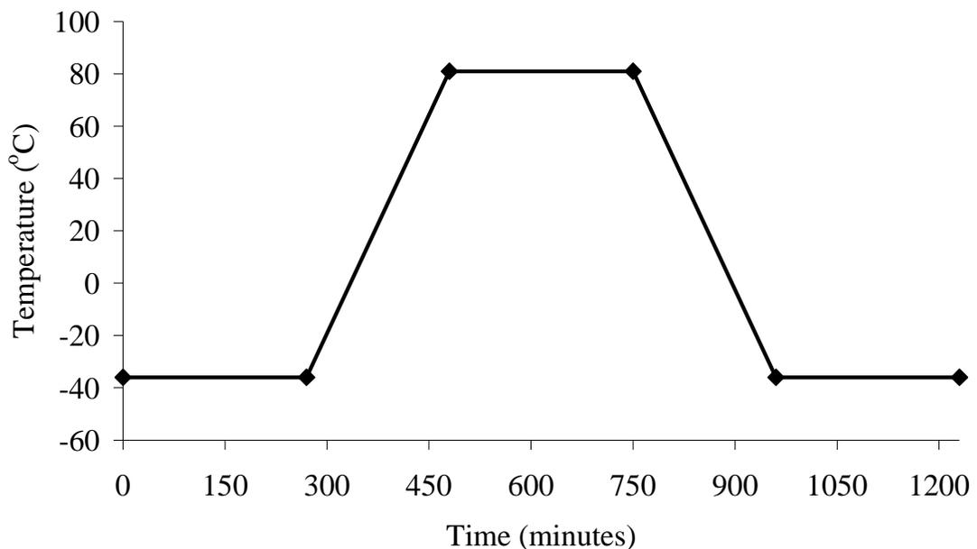
**Figure 4-2 Qualification temperature cycle**
