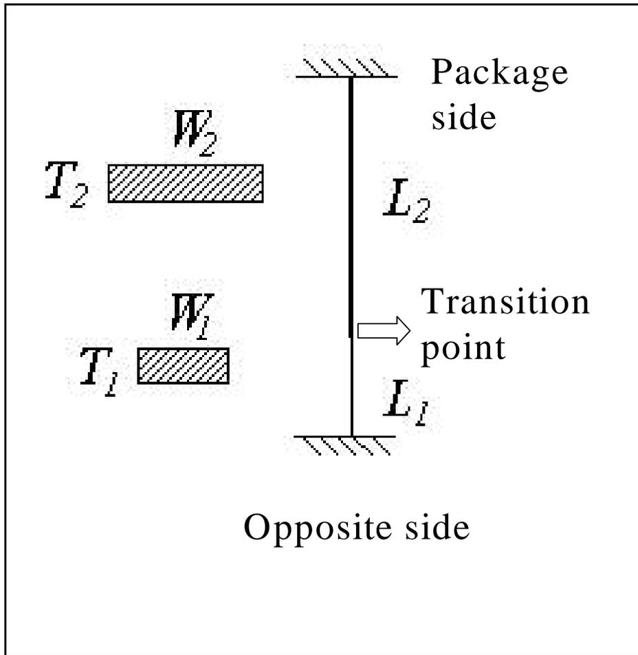
Figure 6-1: Interconnect dimensions for Insertion mount components
