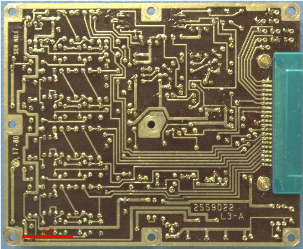
Figure 3-3: This photo shows the solder side of board #2, identification number 2559022. Visual inspection was performed on this board.
