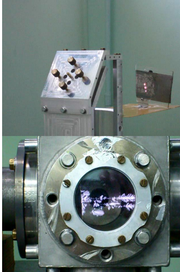
Figure 1.22 The terahertz breakdown observed in the air and in the argon filled chamber.
