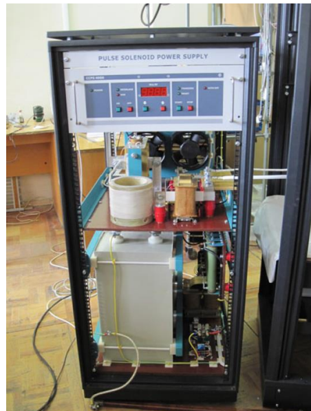
Figure 1.11 (a) Time dependence of the pulsed solenoid current, (b) Pulse solenoid power supply
