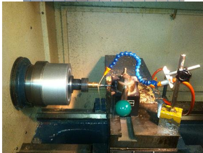
Figure 1.17 The manufactured resonators and the machining setup used in the manufacturing process.
