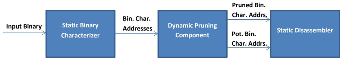
Figure 2.5: The disassembler with the dynamically assisted component inserted
