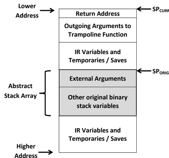
Figure 3.3: The memory stack layout after executing a trampoline call
