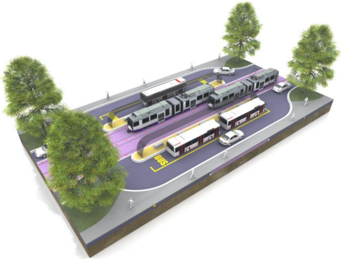
Illustration 61 Design Example 1: 2 lanes. Improvement on public transit facilities, pedestrian facilities and planting. Incorporated with the Purple Line.
