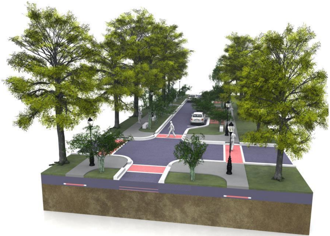
Illustration 68 Design Example 2: 1 lane with parking lane. Improvement on pedestrian facilities, green infrastructures and planting.
