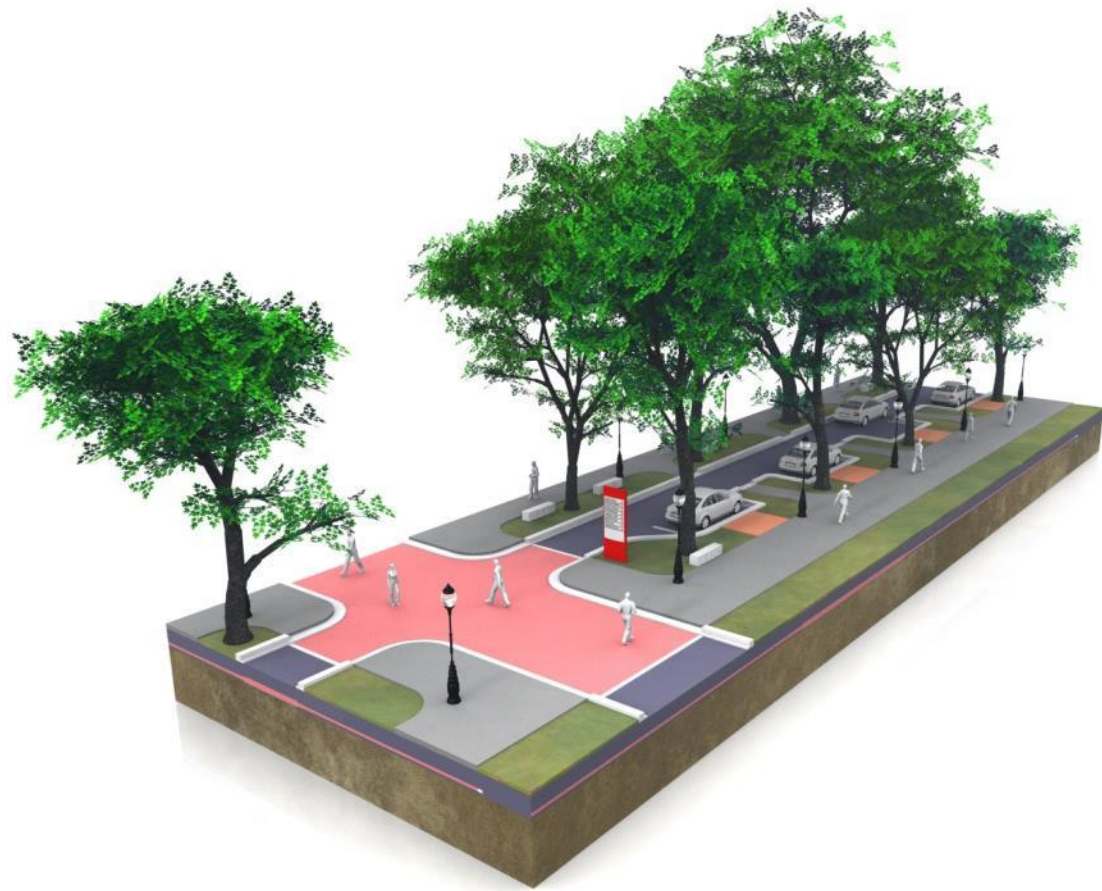
Illustration 59 Design Example 3: 1 lane with parking lane. Improvement on pedestrian facilities and planting.
