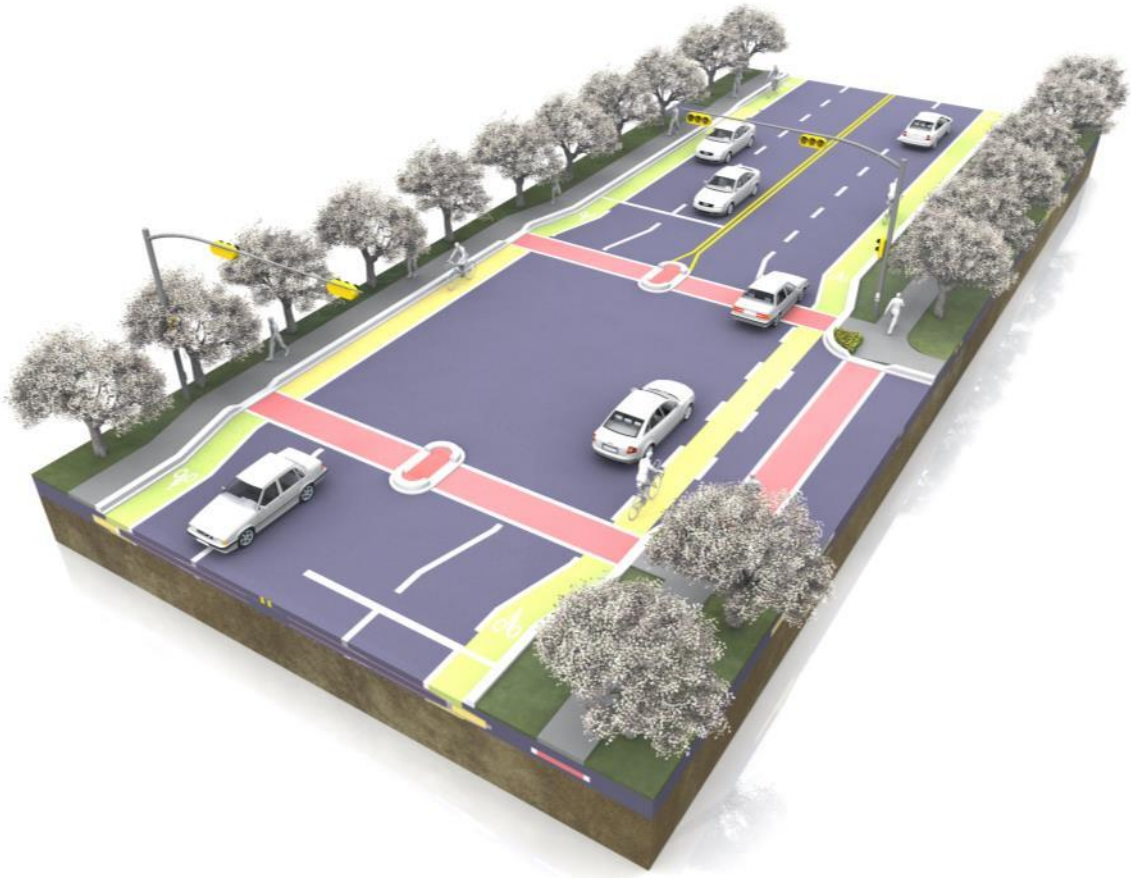
Illustration 54 Design Example 3: 4 lanes with/without extra lane. Improvement on pedestrian facilities, biking facilities and planting.
