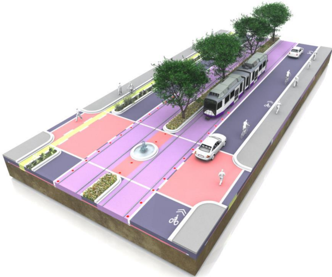
Illustration 56 Design Example 5: 2 lanes. Improvement on biking facilities, pedestrian facilities, green infrastructure and planting. Incorporated with the Purple Line.
