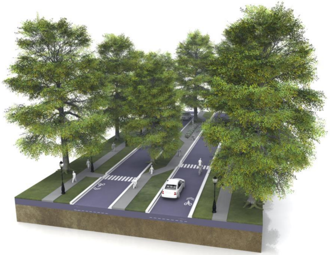
Illustration 67 Design Example 1: 2 lanes with median. Improvement on biking facilities, pedestrian facilities, green infrastructures and planting.
