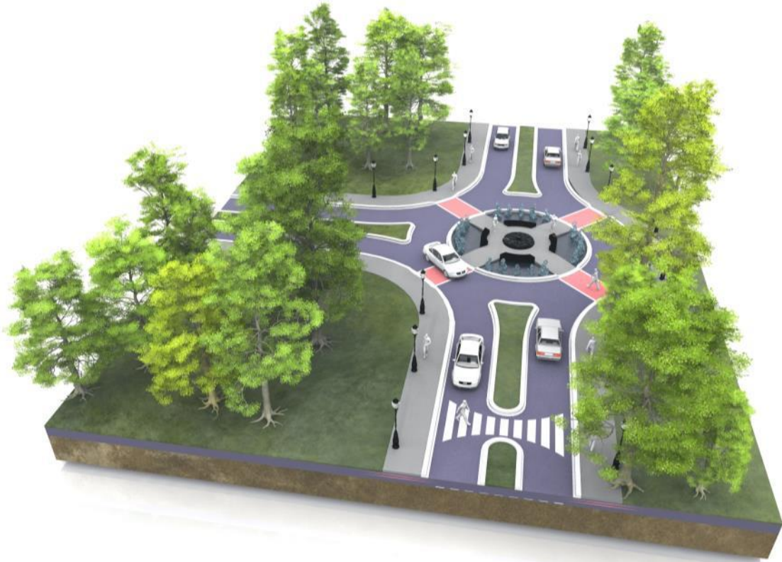
Illustration 55 Design Example 4: 2 lanes with median. Improvement on pedestrian facilities, green infrastructure and planting.
