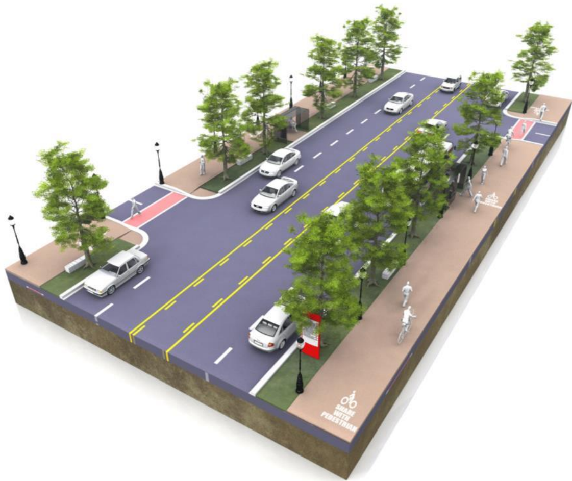
Illustration 53 Design Example 2: 4 lanes with central turning lane. Improvement on pedestrian facilities, biking facilities, public transit facilities and planting.
