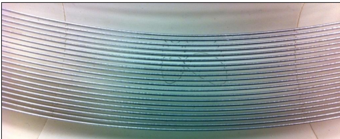
Figure 13 – Coil Layer with Proper Air Gap Between Windings
