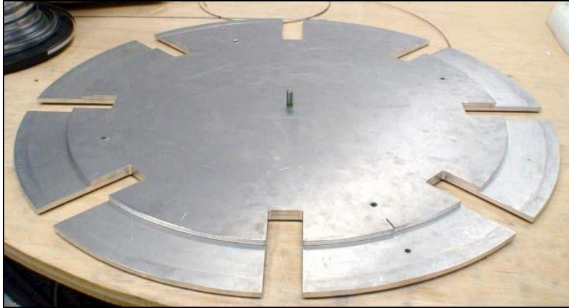
Figure 7 – Spool Used to Manufacturer Coil Layers
