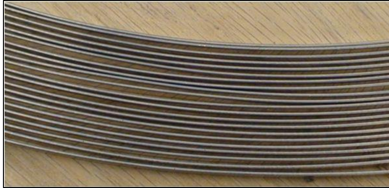
Figure 10 – Undesirable Winding-to-Winding Contact as a Result of No Heat Treatment
