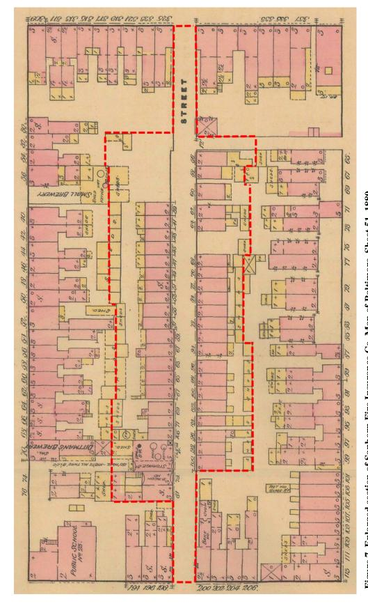
Figure 7. Enlarged section of Sanborn Fire Insurance Co. Map of Baltimore, Sheet 51, 1880. Note: study block outlined. Pink = brick structure and yellow = wooden structure.
