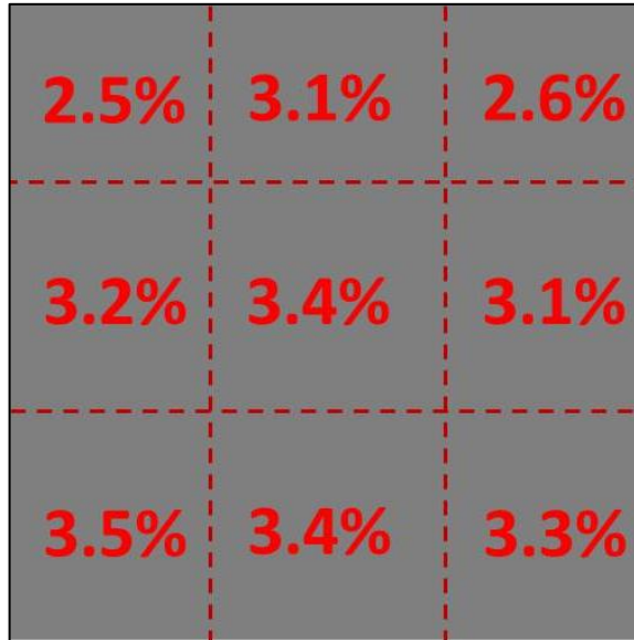
Figure 33. Oxygen Concentration in CAPA Environment, with Cone Heater at 50 kW/m 2 and 200SLPM of N 2
