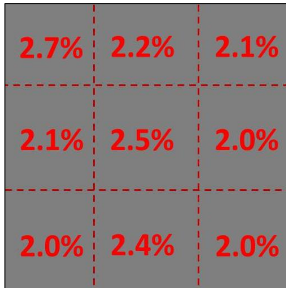
Figure 30. Oxygen Concentration at the Sample Surface with CAPA, Cone Heater is Off
