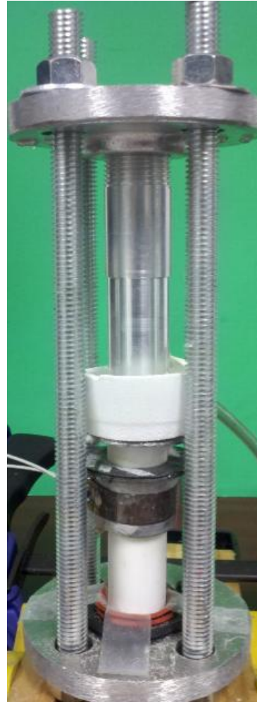
Figure 2-2. Prototype design of thermoacoustic flashover detector.
