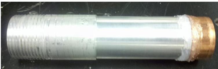
Figure 2-11. Cold heat exchanger connection to aluminum open-ended pipe.
