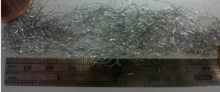
Figure 2-5. Strip of steel wool cut from initial sample to form the stack.
