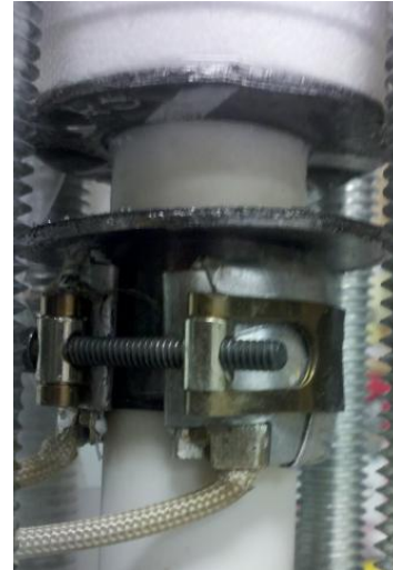
Figure 2-10. Close-up of stack holder post-assembly
