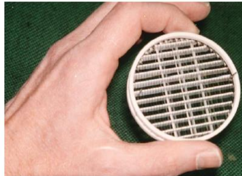
Figure 1-6. Electric-resistance hot heat exchanger used at Los Alamos [8].
