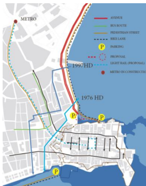
Figure 33 Existing Transportation System by author
