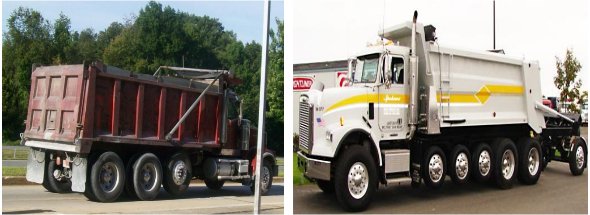
Figure 2.1: 4-axle Dump Truck with Lift Axle (L) and 7-axle Truck with Lift Axles (Ref: maxleairride.com ) (R)
