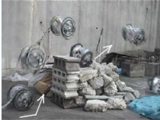
Figure 3 Leg-in-Rotor rescue robot uses pneumatic actuators to jump over debris [5]
