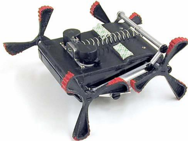
Figure 2 The Mini-Whegs 9J is capable of running and jumping locomotion [8]
