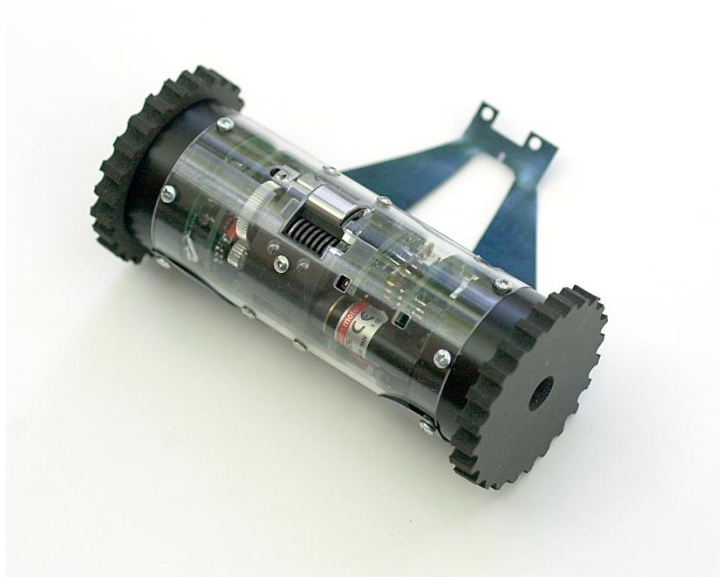
Figure 5 Scout robot similar to that shown in [9] where the spring foot is located to the rear [11].
