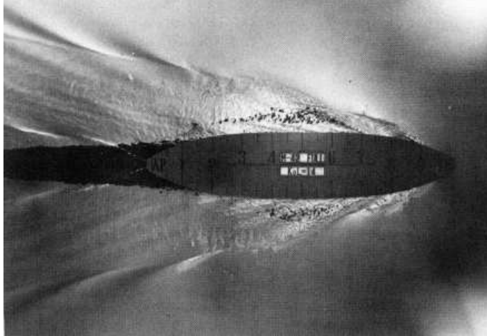
Figure 2.4: Wave patterns around a fine ship model with the draft of 0.105 advancing at F_n = 0.267 . The water surface, covered with an aluminum powder film, is split near and behind the model.
