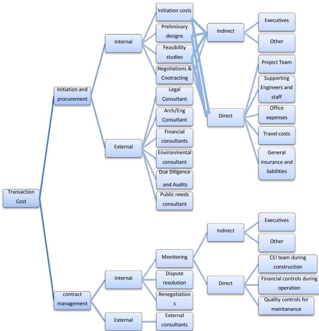
Figure 10: Transaction Cost Breakdown Structure
