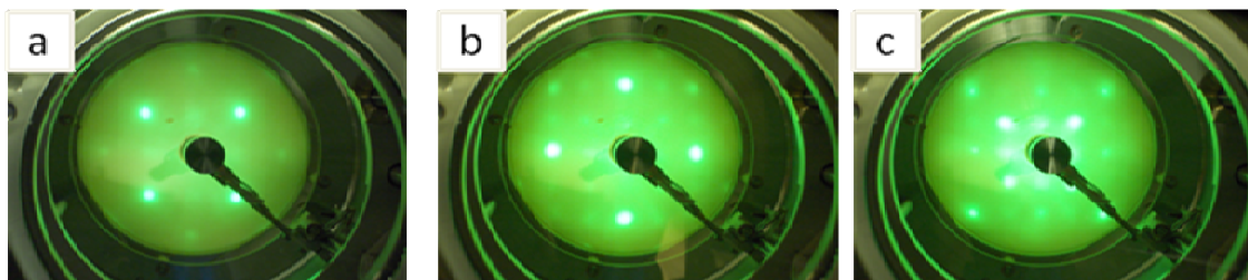
Figure 5.5 Low energy electron diffraction (LEED) images on an ultrathin Fe film grown at 400 °C on MgO (001) substrate. The diffraction energy for each of these images is (a) 40 eV, (b) 65 eV, and (c) 78eV. These images show the bcc crystalline structure of the Fe film, indicating a good epitaxial growth.
