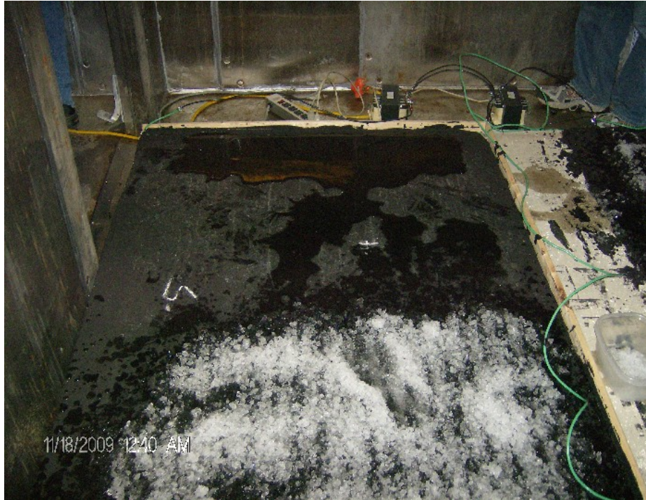
Figure 28. The large panel after an hour and a half. Notice the puddle of water forming from melting of the ice. The control in the plastic container on the right has shown no signs of melting.
