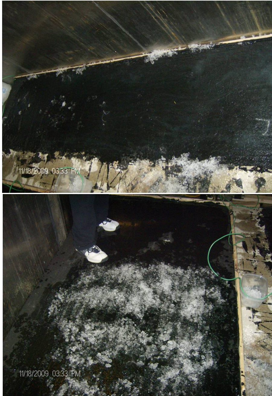
Figure 30. The smaller test section (left) has almost all the ice melted at the 4 hour mark. The large panel (right) at the same time has much of the ice melted off the pavement.
