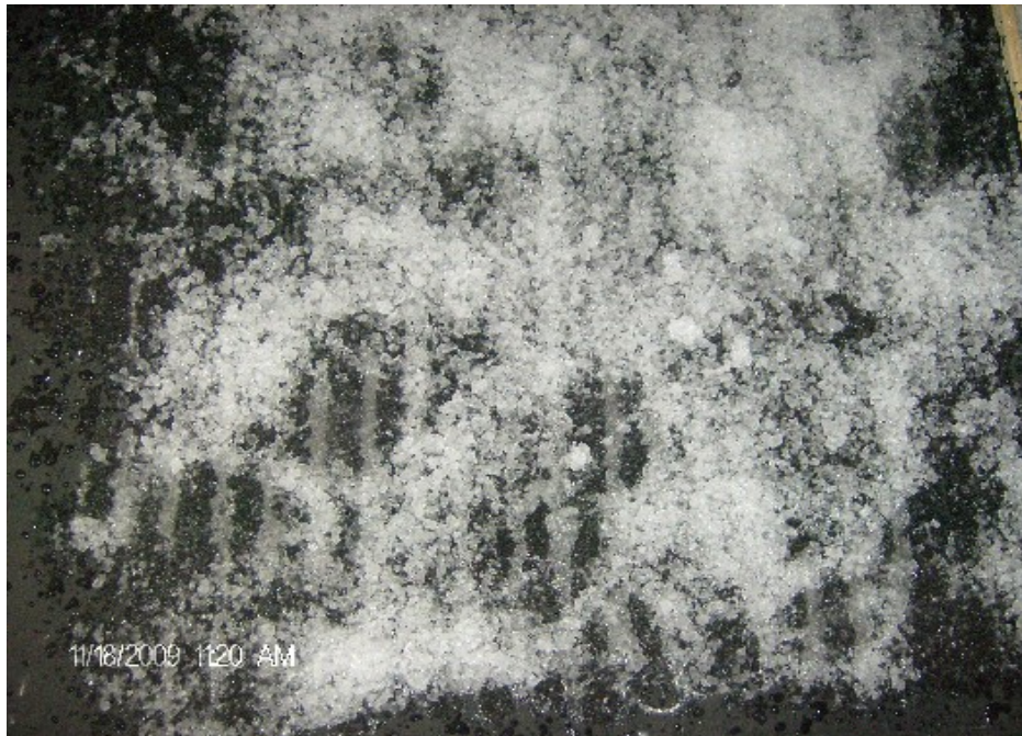
Figure 27. The large panel after 15 minutes of run time. Notice the banding pattern of melting caused by the wire spacing.
