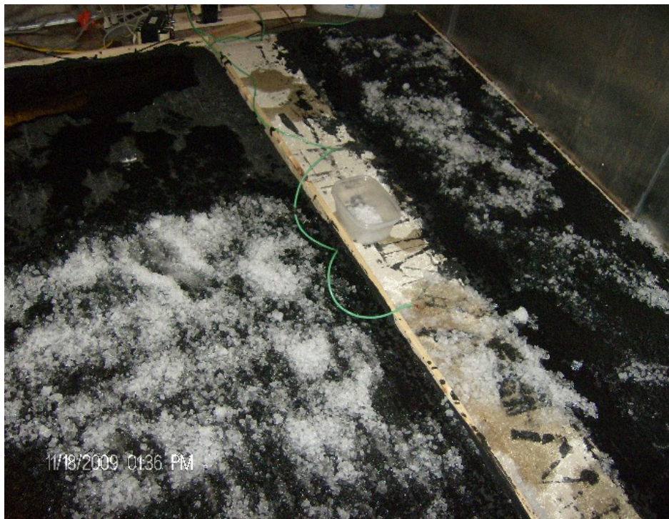
Figure 29. Both panels after 2 hours. The smaller panel has almost melted all the ice and the larger panel has melted a significant portion shown by the puddle forming at the top left of the photograph.
