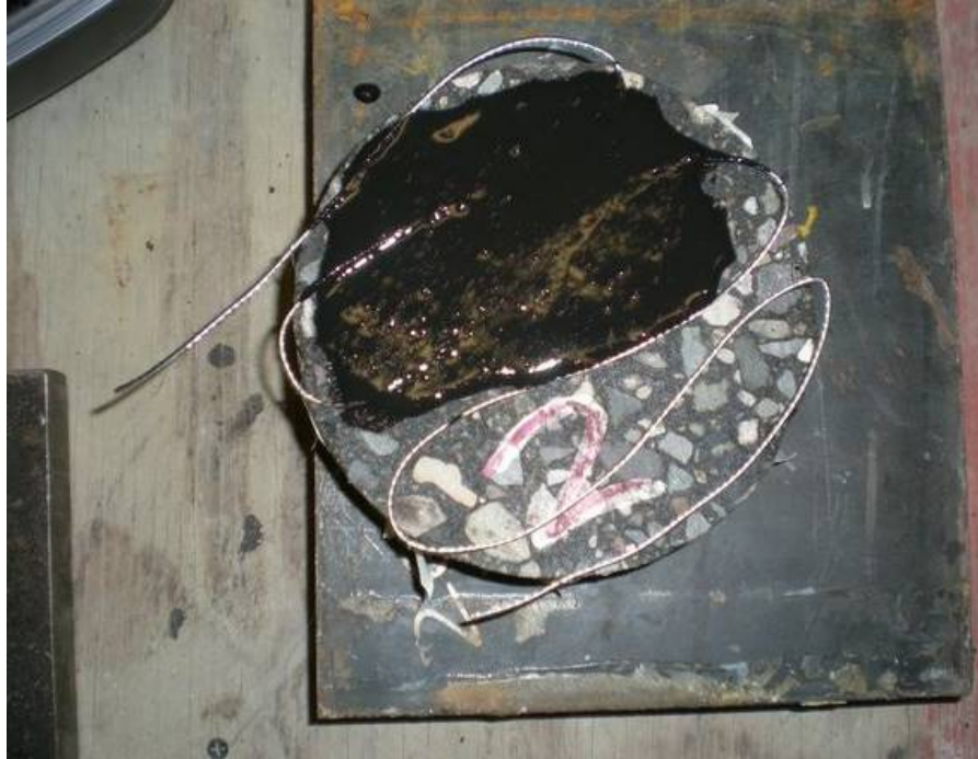
Figure 5. A puck being covered with a thick layer of sealant to cover the wires.
