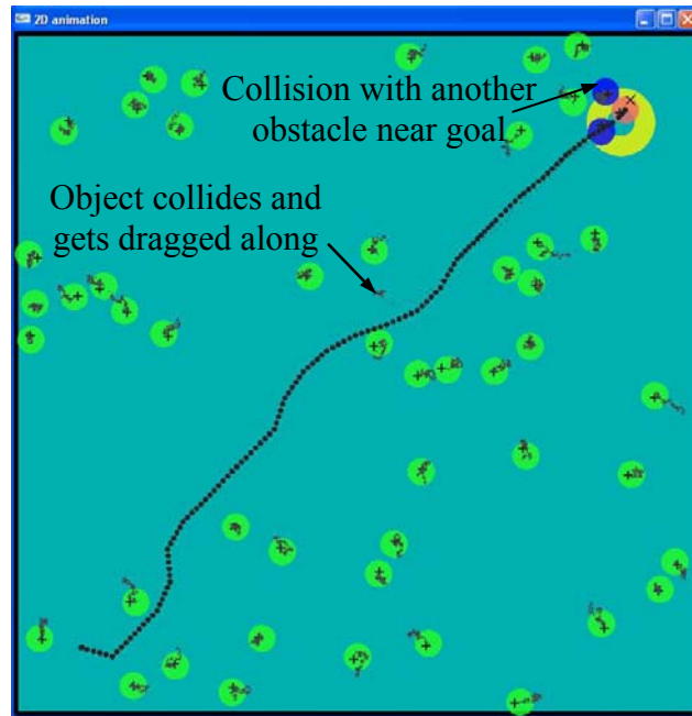
Figure 4.15: Collision and dragging of obstacle in a crowded scene where the relative rate of change in free C -space is quite high
