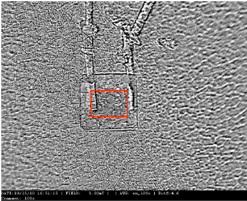
Figure 28, Kerr microscope image of a 50x50 \mu\text{m} FeGa/PZT device with a magnetic domain boxed in red, taken at 100x.
