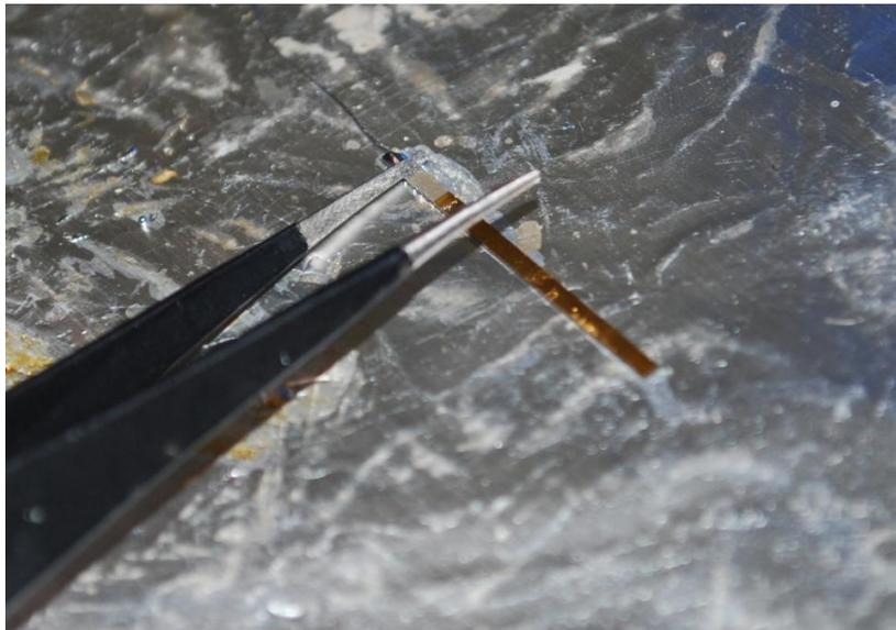
**Figure 3.12 In/Sn solder reflowing of piezoelectric beam to secure constantan wire.**
