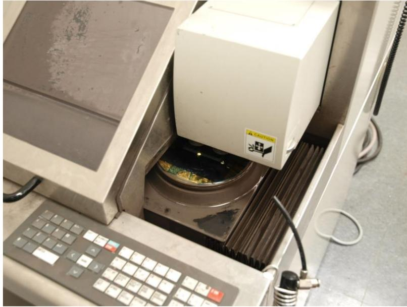
**Figure 3.9 Dicing of piezoelectric sheet and carrier wafer on Disco DAD321 dicing saw.**
