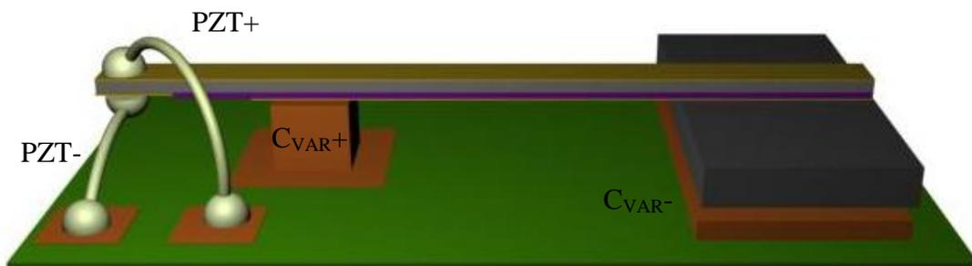
**Figure 6.2 Concept rendering of volume reduction by using a Cu mounting peg.**
