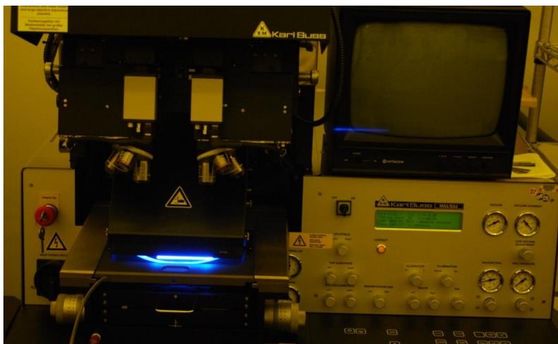
**Figure 3.6** KMPR exposure sequence using LAMPTEST on Karl Suss MA-6 aligner.
