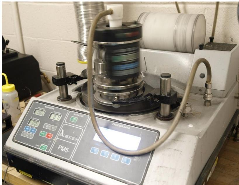
**Figure 3.21 Lapping of tungsten blocks on Logitech PM5 tool.**
